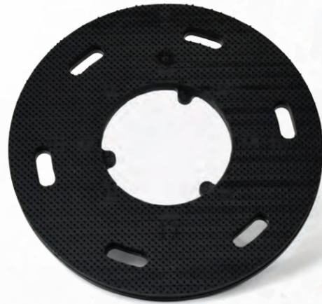
The **SURE-LOK® System** is an exclusive Malish design for use on dual and high speed (300 rpm) machines. The SURE-LOK® face combines our MIGHTY-LOK® molded polymer pad gripping material with a foam cushion to absorb vibration and a stiff plastic backing to stabilize the unit. SURE-LOK requires the use of the high speed riser. Available in 17" and 20".
